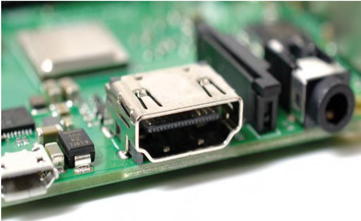
Fig. 3.10 The Raspberry Pi's HDMI port
