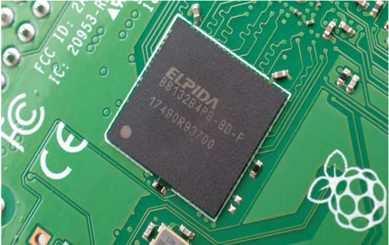
Fig 3.3 The Raspberry Pi's random access memory (RAM)
