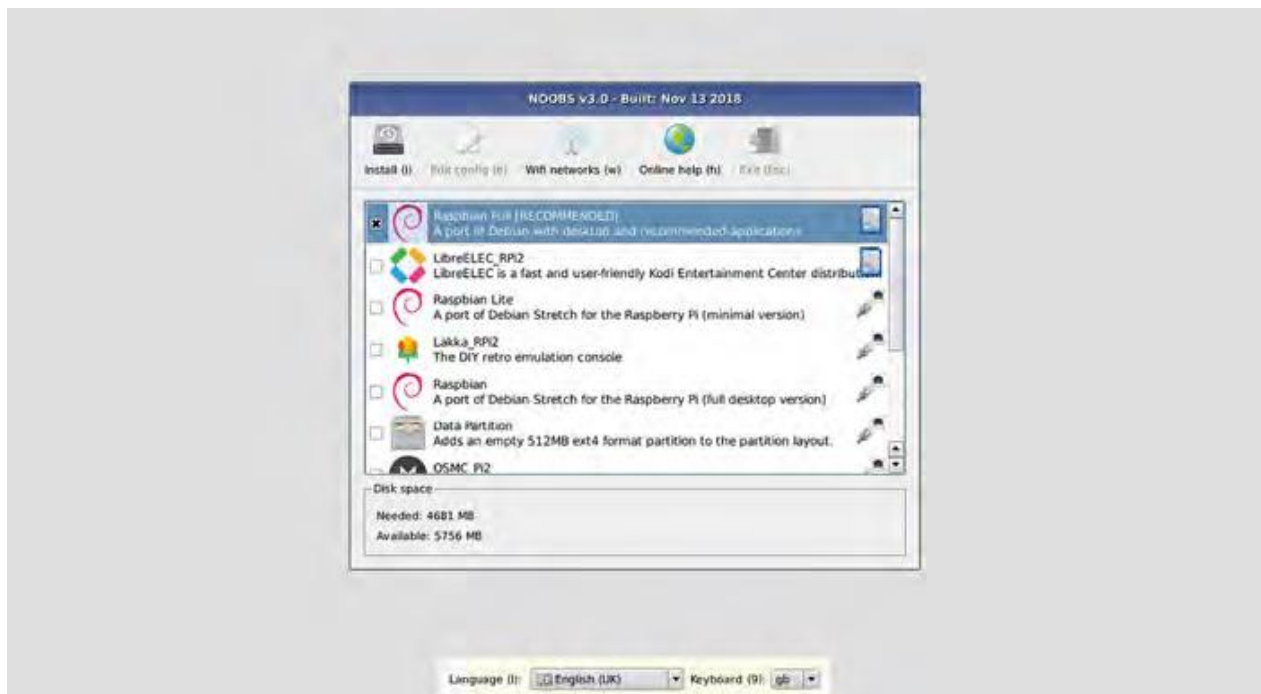
Fig 4.3 The NOOBS menu with Raspbian operating systems installed
