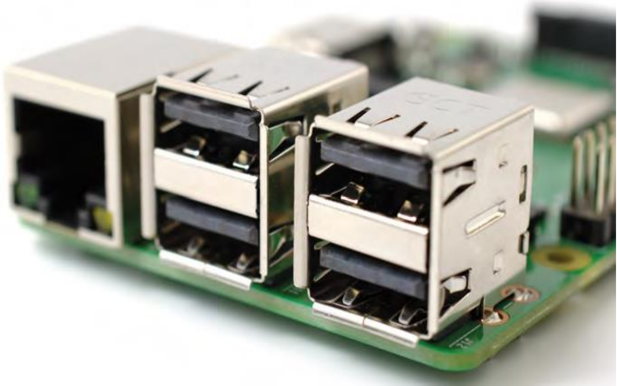
Fig 3.6 The Raspberry Pi's USB ports
