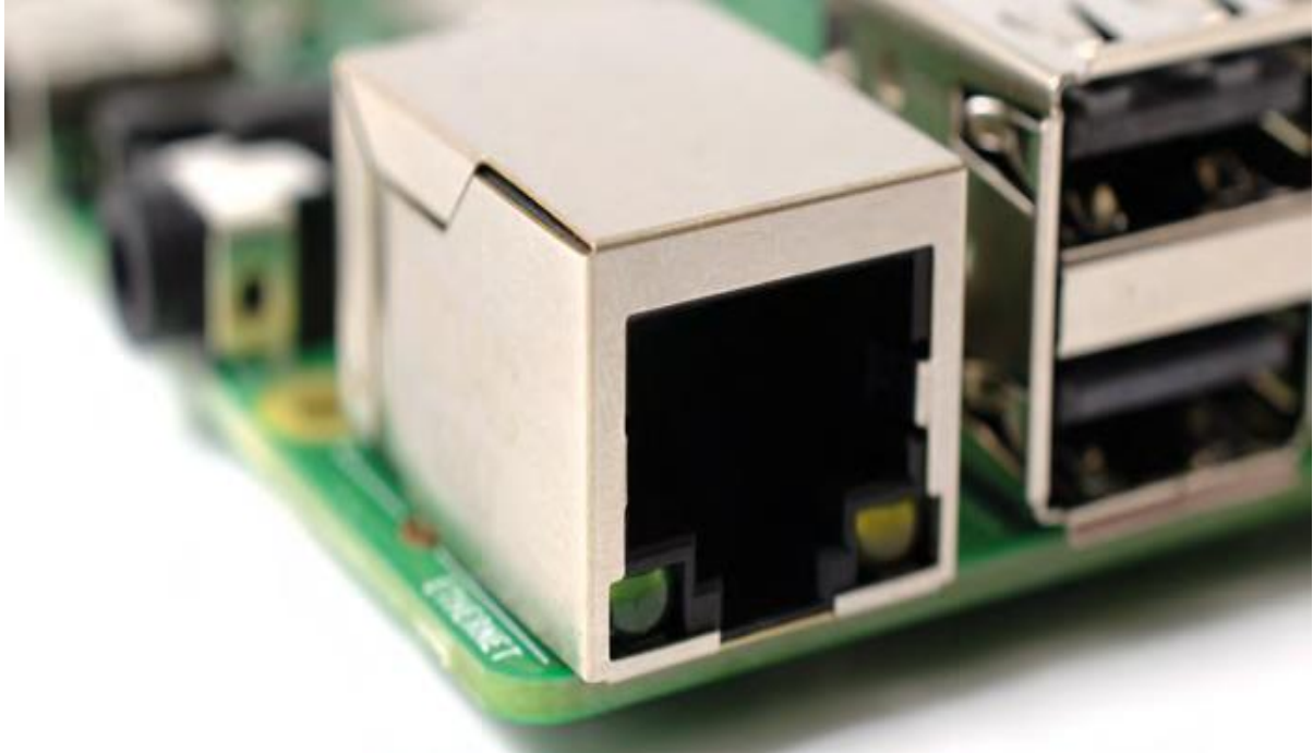
Fig 3.7 The Raspberry Pi's Ethernet port
