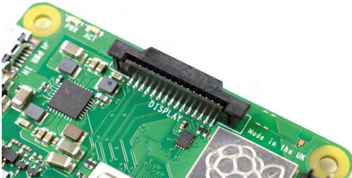
Fig 3.12 The Raspberry Pi's display connector (DSI)
