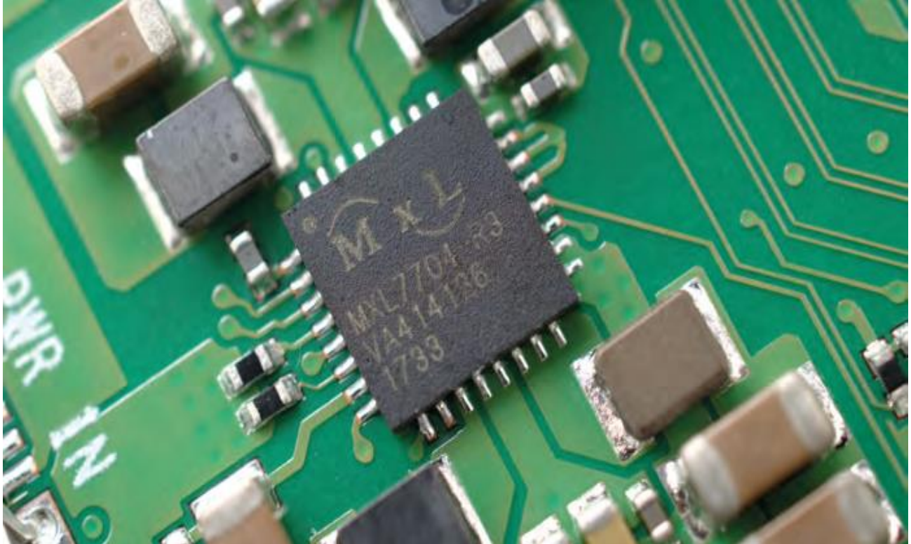
Fig. 3.5 The Raspberry Pi's power management integrated circuit (PMIC)
