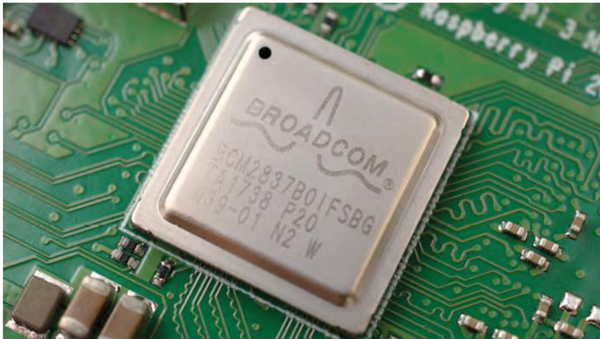
Fig 3.2 The Raspberry Pi's system-on-chip (SoC)
