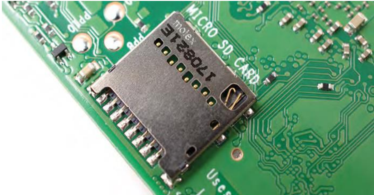
Fig. 3.13 The Raspberry Pi's microSD card connector
