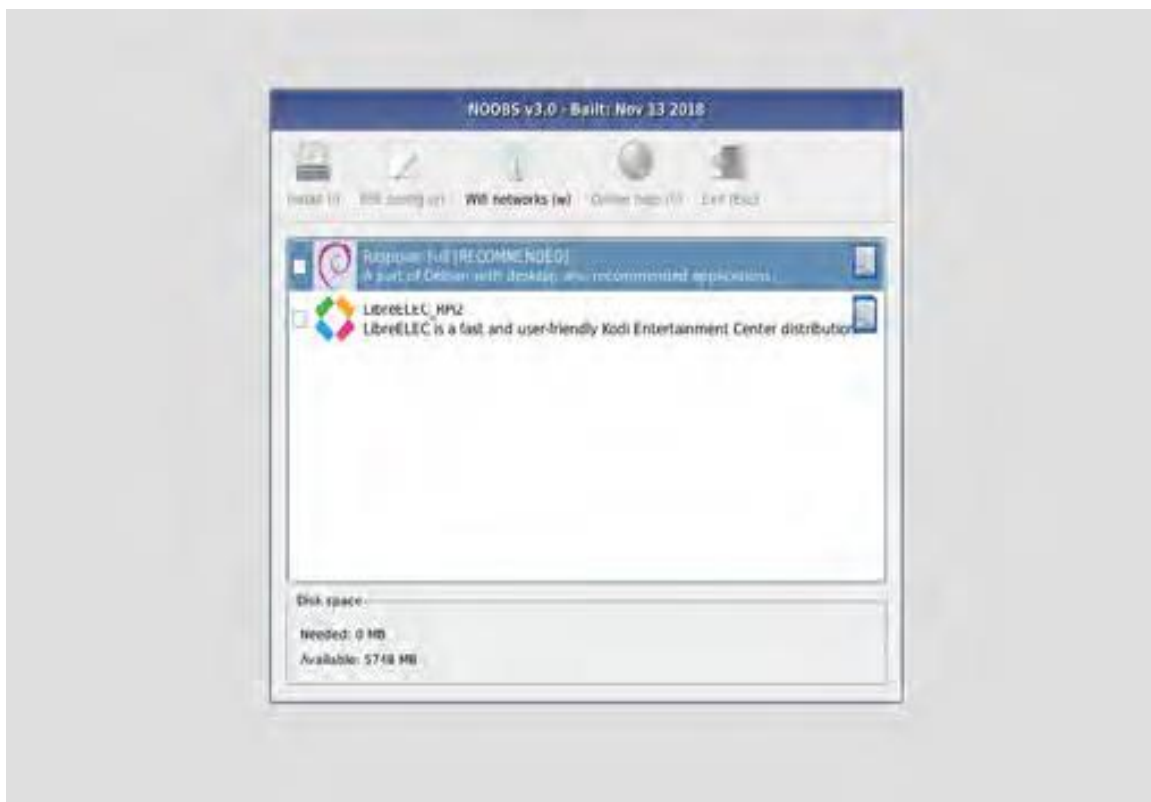
Fig 4.2 The NOOBS menu without any operating systems installed
